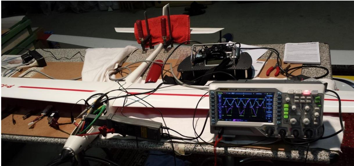
Motor: AXi 2820/10    Poolzahl: 12     $k_v = 13000 / 11.4 = 1100 \text{ RPM/V}$      $R_{2w} = 20.5 \text{ m}\Omega$
